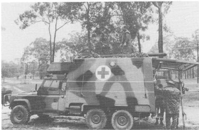
The new PERENTIE ambulance during trials. Note the rear door (no, its not supported by the litter.)
